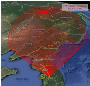
**Figure 2. TPY-2 radar coverage** (aka “fan”) is shown in red. Any object with a radar cross section of more than one square meter can be detected and tracked by the TPY-2 radar, whose notional location is roughly 100 km north of the current THAAD deployment site.
