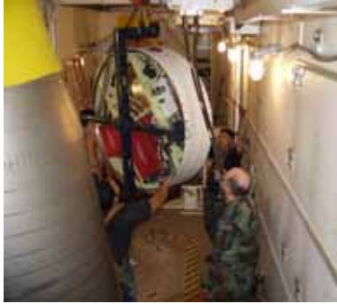
Malmstrom maintenance at work replacing a guidance system
