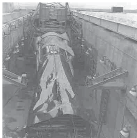
An Atlas E after loss of pressurization.
