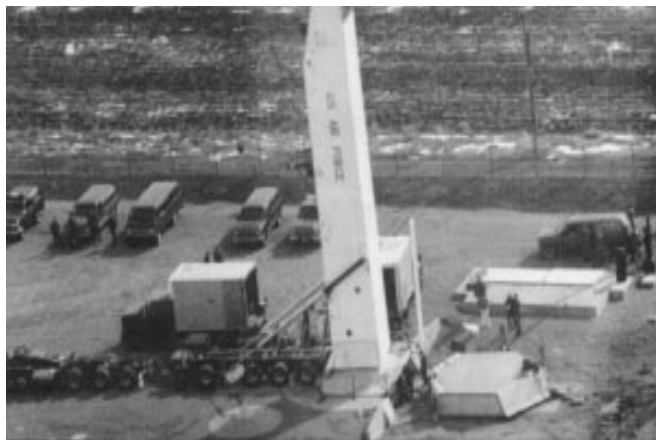
Minuteman Transporter-erector and other vehicles on site during missile change
